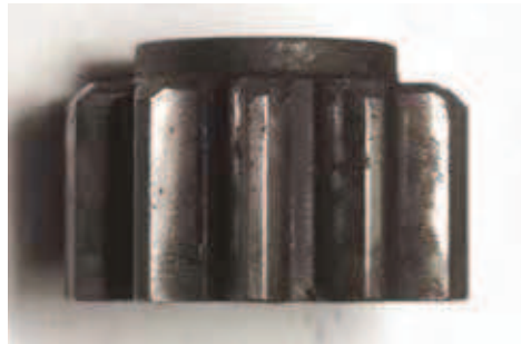
Normal wear marks showing over 3/4 of the drive surface being used.
