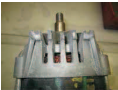
Mounting ear completely broken off
